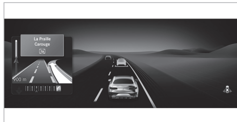
Active Distance Assist DISTRONIC indicator on the assistant display (example)
